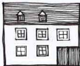
Loft conversion incorporating gabled dormers.
